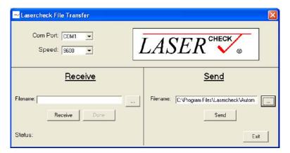
File Transfer Software Configured to Send Calibration / Setup File
