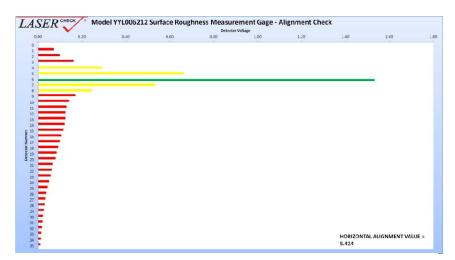
Typical Spreadsheet Alignment Curve Showing Specular on Detector 6
