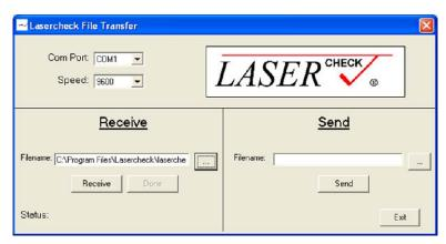
File Transfer Software Configured to Receive Saved Measurements
